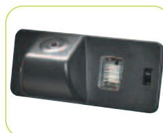
IPCVS543D • BMW X3/X5 2005-up/ X6 2009-up, 3Series 2009 and 5 Series Sedans • CCD format - 170° Angle • Replaces license plate light • 1/3" Sony color camera
